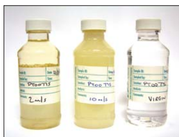
Lip Seal Test: Oil sample bottles for lab analysis.
